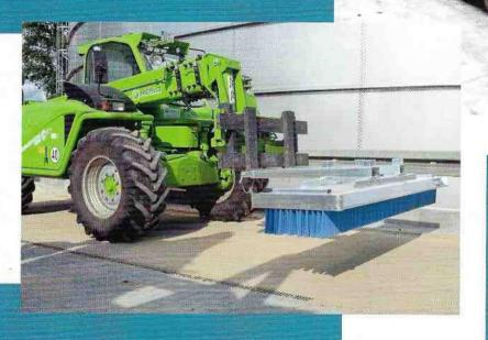
Construction: sweeping construction sites, spreading sand and gravel, sand back-filling without generating dust and damaging the subsoil
